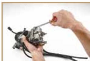
Step 1: Remove the carburetor side cover and the float bowl.
